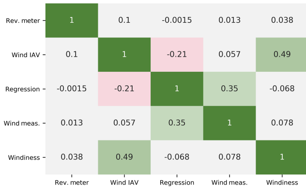
Figure 6. Correlation coefficient heat map between operational AEP uncertainty components, as calculated from each pair of AEP uncertainty components across the 472 wind plants considered in the analysis. Note that “Rev.” denotes “Revenue”.
