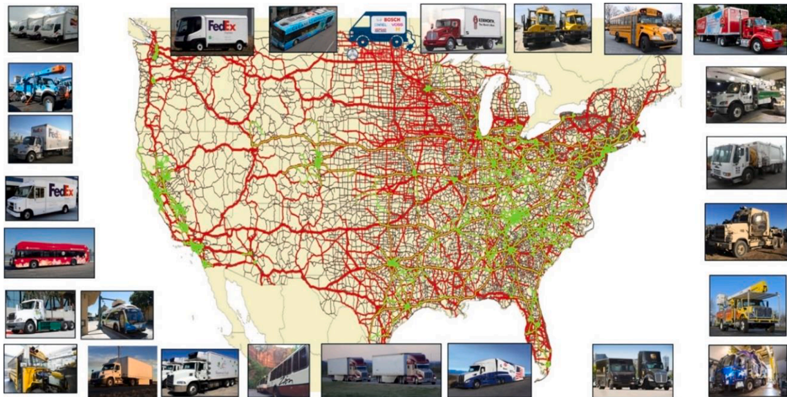
Fig. 1. Map showing freight volumes (red) along major U.S. roadways and Fleet DNA data coverage (green) along those routes, as well as the involved vehicle vocations. (For interpretation of the references to colour in this figure legend, the reader is referred to the web version of this article.)
