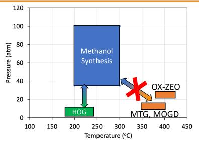
Similar process conditions offer the opportunity for process intensification to enable direct syngas-to-fuels through methanol in a single reactor
