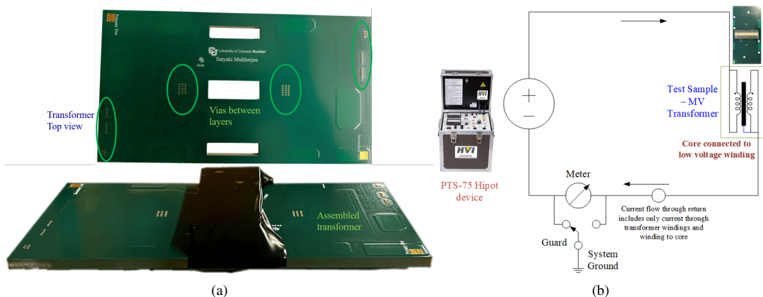
Figure 6: MV transformer and hipot test setup: (a) Fabricated planar MV transformer: PCB winding top view and assembly, and (b) circuit diagram of the guarded hipot test setup used to verify the isolation capability of the MV transformer.
