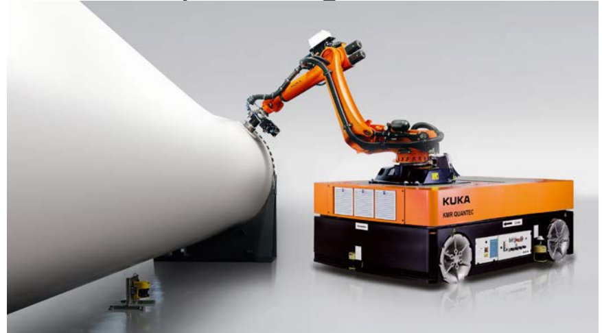
Kuka robotic polishing mobile platform Source: Kuka
