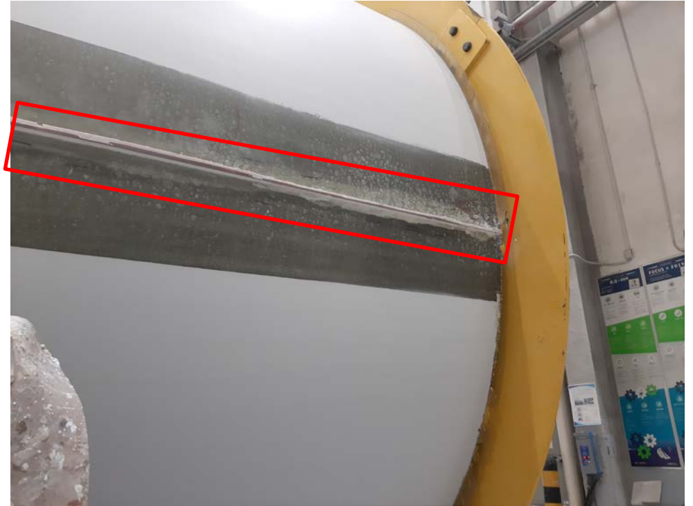
Preoverlaminated blade root Source: LM Wind
