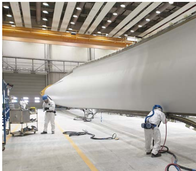
Flashing trimming Source: LM Wind
