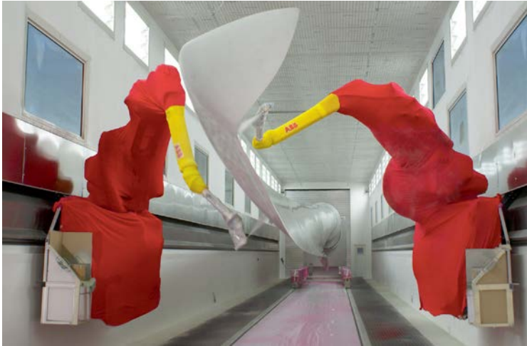
ABB blade painting robots Source: ABB
