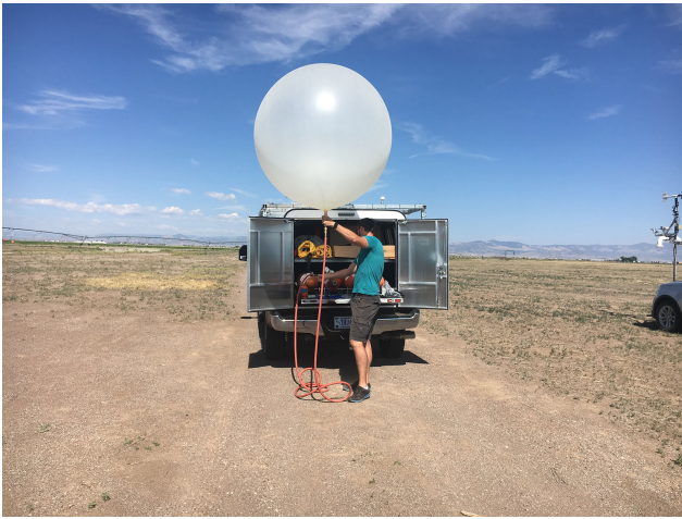
Figure 4. A radiosonde launch at Leach Airfield by Dr. Sean Waugh. Photo credit Dr. Sean Waugh, NOAA/NSSL.
