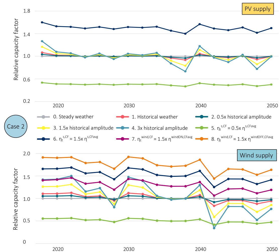
Fig. 4. Case 2 - Fluctuating weather scenarios 0–8 with relative capacity factors for PV a and Wind supply from 2018 to 2050. a N.B. Scenarios 7 and 8 do not fluctuate the PV capacity factor and correspond to Scenario 1.
