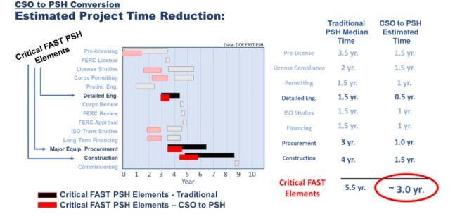
Usage of CSO Tunnels could reduce Estimated FAST PSH Time Elements by ~ 40% to 50%
