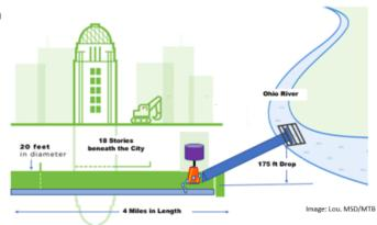
55M Gallons of water falling 175ft has the potential to produce approximately 24 MWh of Energy
