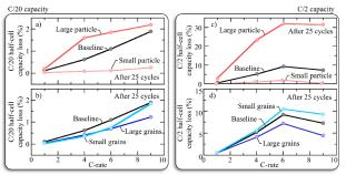
Above are results from all simulations. The left column computed capacity loss by comparing the C/20 discharge capacity after formation and after 25 cycles. The right column is the same calculation but using a C/2 rate. Parts a) and c) compare the geometries with varying secondary particle size and b) and d) compare the geometries with varying grains.
