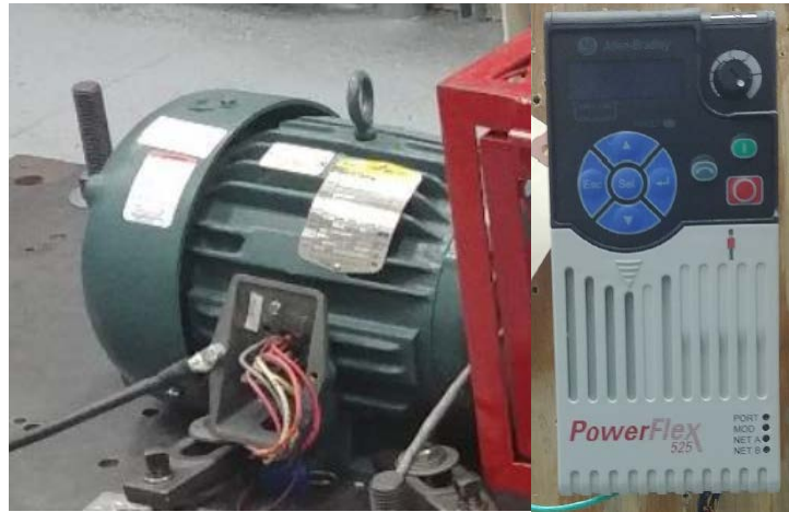
Figure 5. Baseline 2-HP induction motor (left), and VFD (right)
