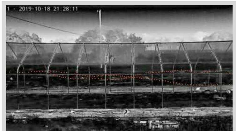
NREL researchers investigated the effectiveness of an ultrasonic acoustic deterrent by using thermal imaging to track the movements (dots in the image) of various species of bats in response to different ultrasonic signals in this open-air flight cage, pictured here. Image courtesy of Brittany Stamp, Texas State University
