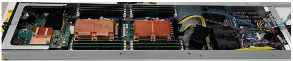
Fans in each node provide primary cooling for low-power components and secondary cooling in the case of a liquid-cooling failure. Image Credit: Chilldyne
