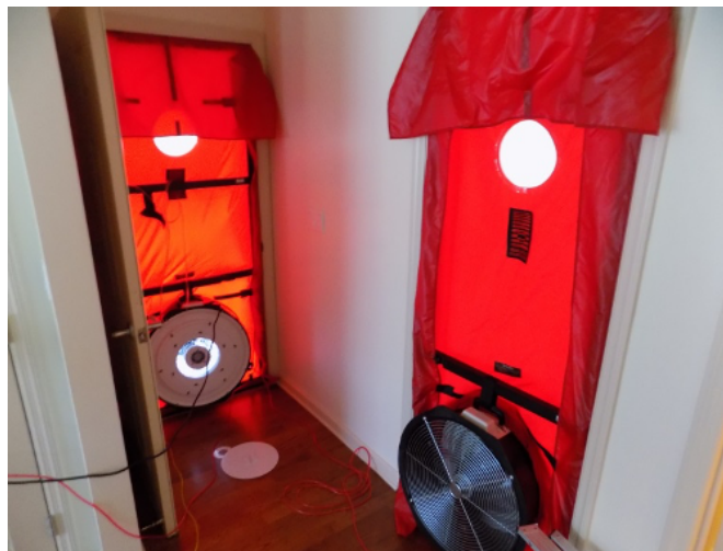
Figure 17. Guarded blower door tests, shown here set up in a single-family home, are similar to standard blower door tests, but use additional fans to isolate specific sections of a building’s facade.
