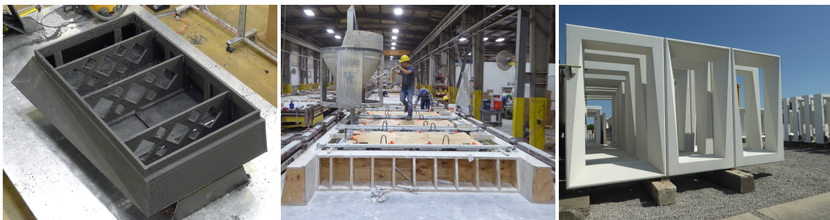
Figure 28. Additive manufacturing has been demonstrated successfully for precast concrete forms of building facades. Avenues to employ advanced manufacturing techniques, such as additive manufacturing, for energy-efficient building envelope components merit additional investigation.
