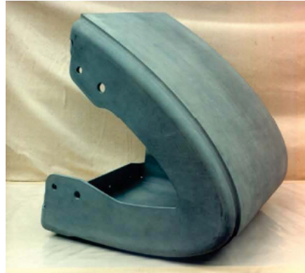
Figure 21. Reinforced carbon-carbon is a graphite-reinforced carbon composite matrix with thermal anisotropy used for the nose cap and wing leading edges of the Space Shuttle Orbiter.
