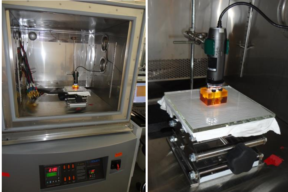
Figure 22. Environmental chamber with USB microscope and membrane sample holder (left), close-up of USB microscope, holder and translation stage (right).
