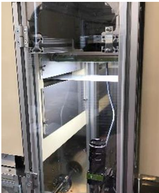
Figure 14. Mainstream prototype inspection system set up on NREL's coating line, here shown inspecting an as-cast membrane.
