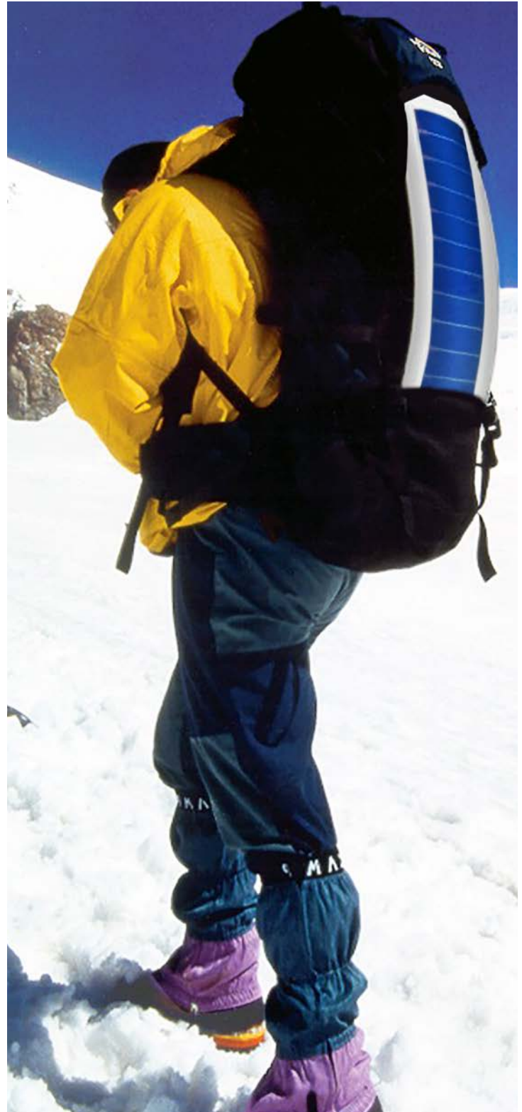
Some photovoltaic technologies, such as thin films, can be flexible and lightweight, so can be used for applications such as aerial transportation or where power needs to be portable. Photo by NREL 13564
