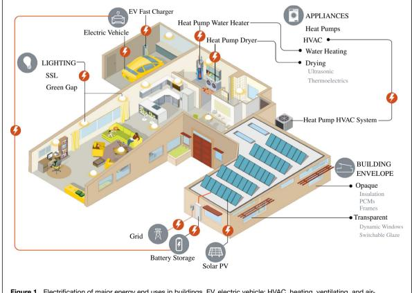
**Figure 1.** Electrification of major energy end uses in buildings. EV, electric vehicle; HVAC, heating, ventilating, and airconditioning; SSL, solid-state lighting; PCMs, phase change materials; PV, photovoltaic.
