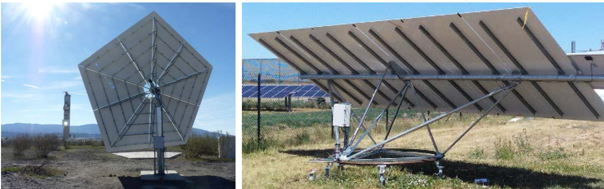
Figure 4. sbp Stellio heliostat (left), and Solar Dynamics SunRing heliostat (right)
