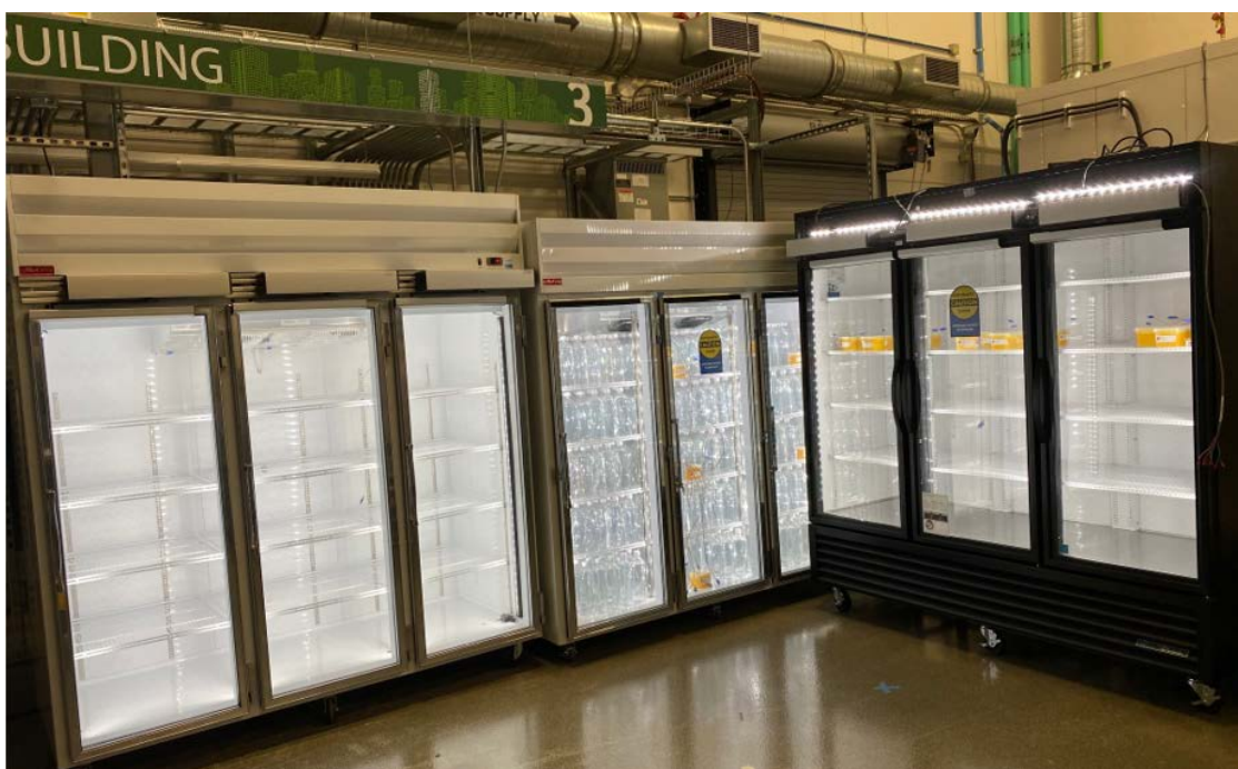
Figure 12. OCL Building Bay 3 with (from left) EE case B, the baseline case (undergoing steady-state testing), and EE case A
