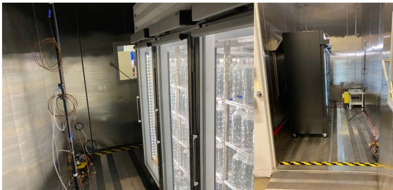
Figure 14. Images of cases in environmental chamber. Left: Baseline case from rear of chamber. Right: EE case A from outside of chamber
