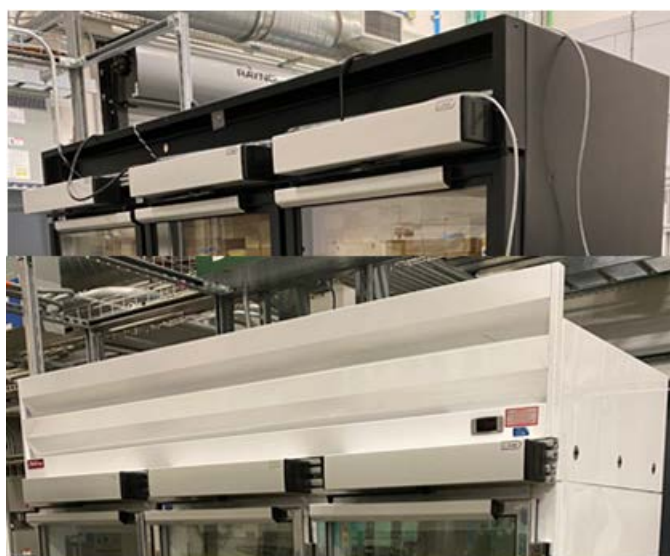
Figure 10. Door actuators mounted to EE case A (top), and the baseline case (bottom)
