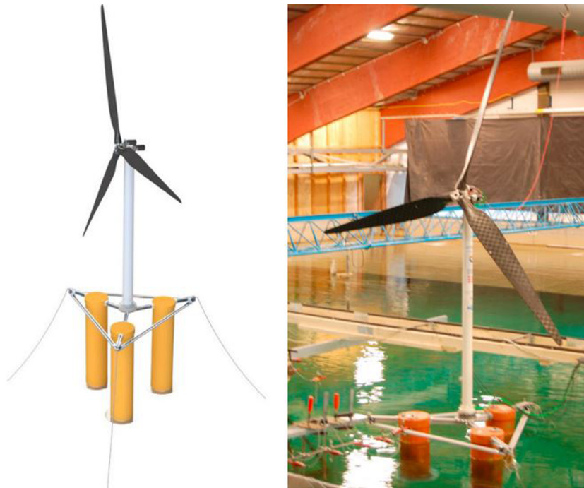
FIGURE 4 The Triple Spar model, left the visualization at scale and right the model in the basin at DHI 122
