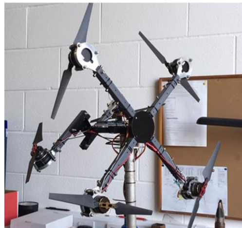
FIGURE 10 Multipropeller actuator, the arrows indicate the thrust direction of the propellers 137
