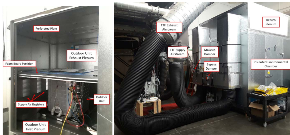
Figure 6. Outdoor unit set inside environmental chamber (left); environmental chamber connected to the TTF airstreams (right)
