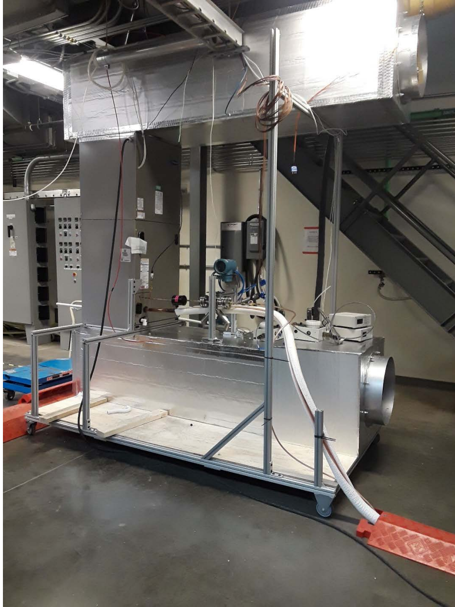
Figure 3. Air-handler (indoor unit), test article mounted on inlet (bottom) and outlet (top) plenums
