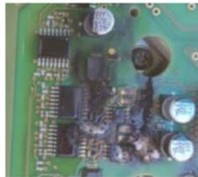
PV inverter boost stage gate driver damaged
