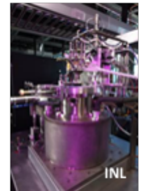
TAP reactor for extracting quantitative kinetic data
