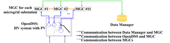
Fig. 1. Overall diagram of the HELICS platform for the peer-to-peer algorithm performance evaluation.
