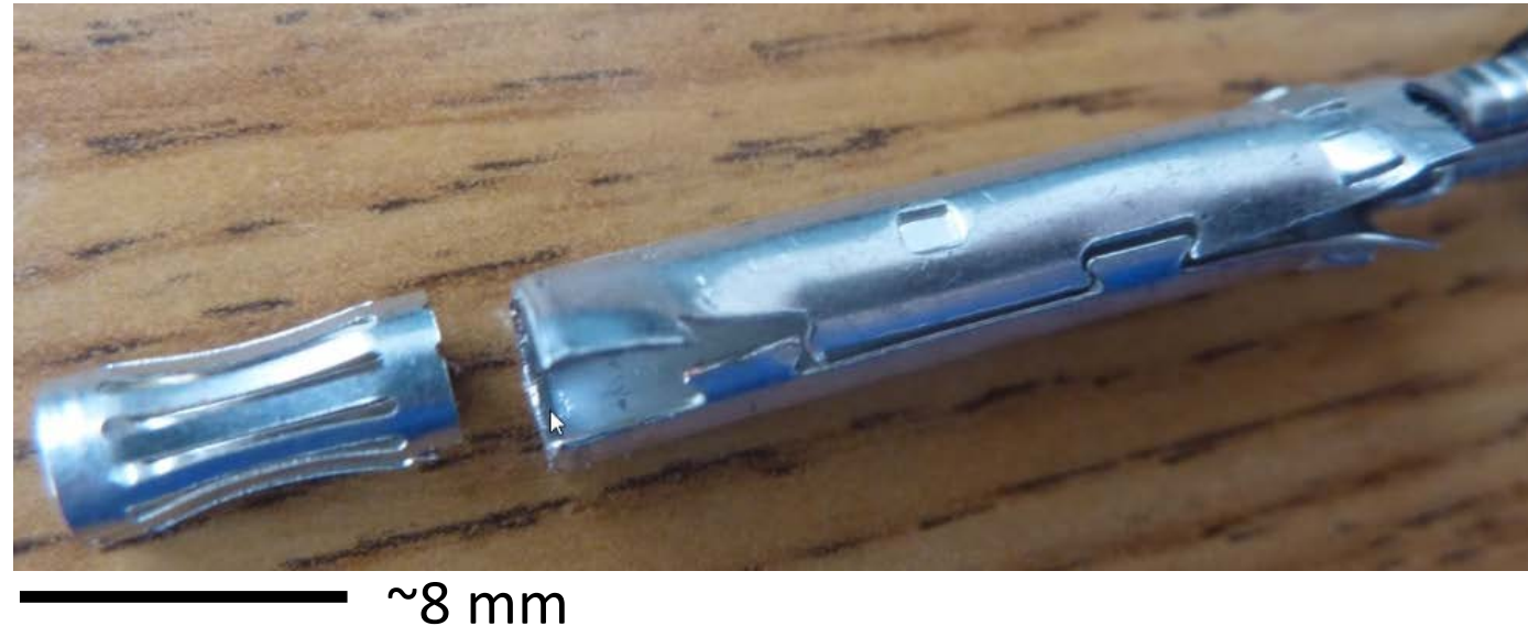
convolute spring, extracted from unaged metal pin
