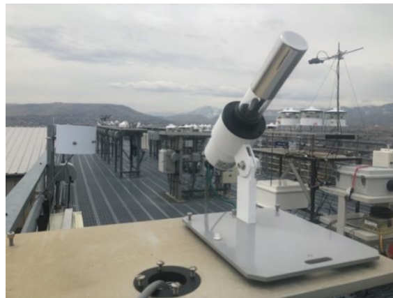
Figure 5. EKO MS-90 deployed at NREL SRRL Baseline Measurement System.
