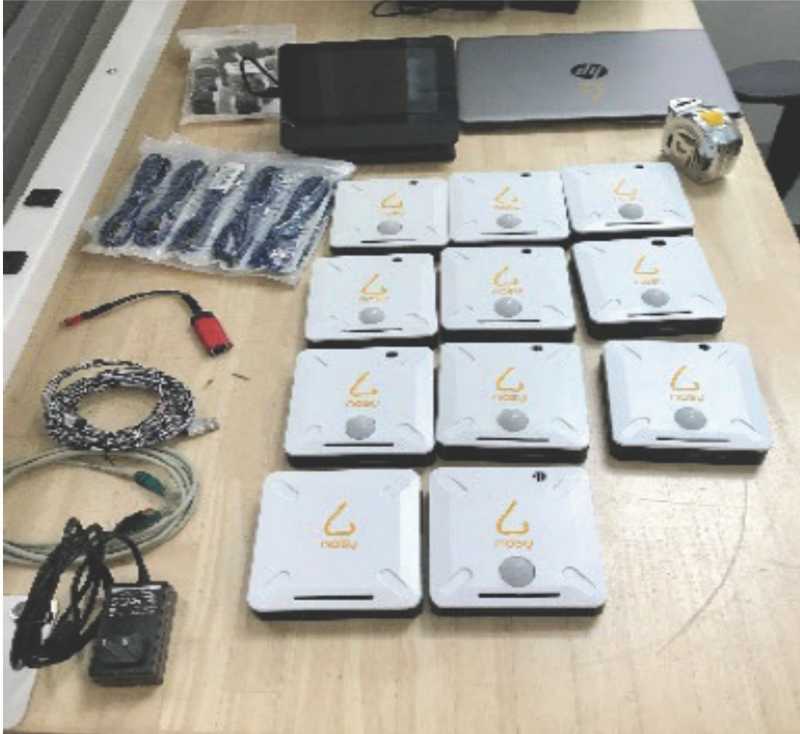
Figure 3. A photograph of the prototype sensor units and touchscreen gateway prior to installation. Each sensor has dimensions of 4"x4"x2". (Image Credit: Amanda Kirkeby, NREL)
