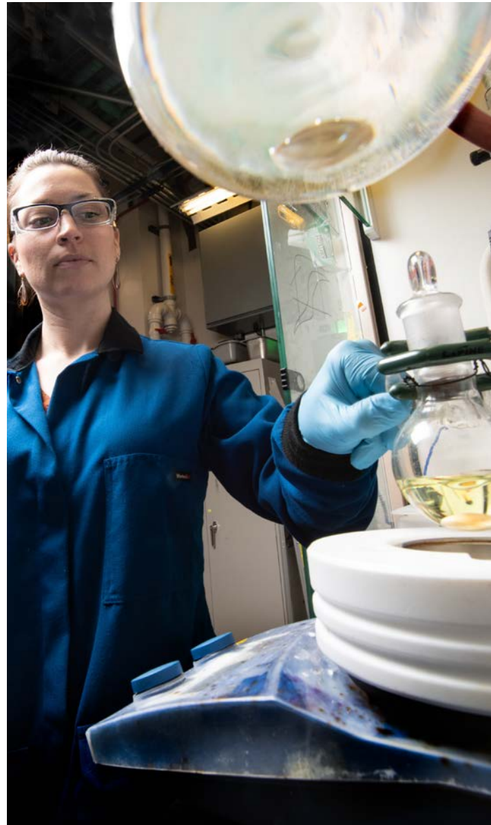
NREL researcher Annalise Maughan purifies materials to be combined with silicon nanoparticles in support of NREL's work on the Silicon Anode Consortium. Silicon-based anodes represent a promising approach to replacing the graphite anode material typically used in lithium-ion cells. Photo by Dennis Schroeder, NREL 61179
