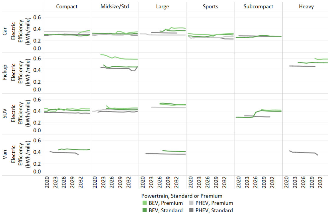
Figure 14. Mid scenario: electric efficiency – BEV and PHEV (charge-depleting mode) powertrains by model year – standard and premium classes
