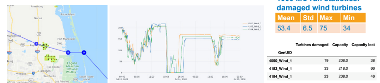
Figure 7: (left) 3 wind plants (heat map) composed of individual wind sites (eight 2-MW turbines per site). Most wind sites had at least one damaged turbine (black dots). (right) Power production at 3 damaged wind plants.
