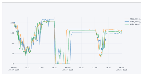
Figure 5: Resulting power outputs as Hurricane Dolly passes by windfarms. Note cutoffs where power drops to zero due to high wind speeds, and that the rated power is less after the hurricane passes due to infrastructure damage.
