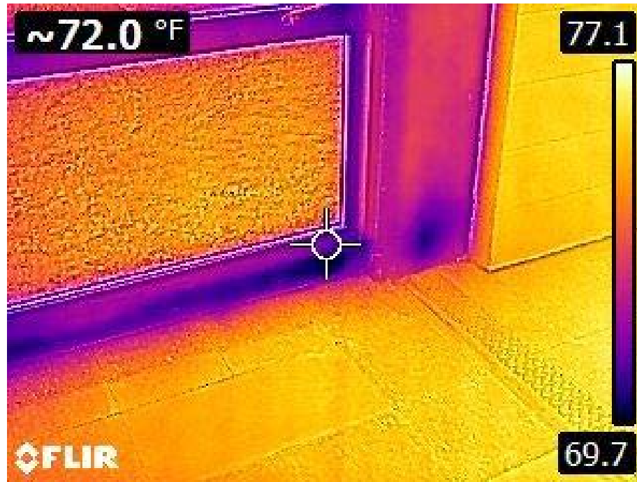
Leakage through a window (this is typical)
