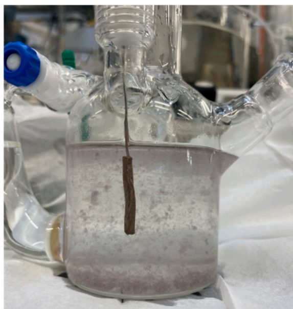
Figure 12. Example of precipitation observed in CaCl 2 after electrochemical corrosion experiments (pictured with CE still immersed in solution; RHE and WE removed).
