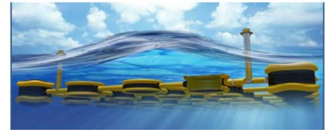
Figure 6: A 75-MW FlexWEC is a cluster comprised of an integrated set of 5-by-15 deformable absorbers with turbine generators in connecting ducts.
