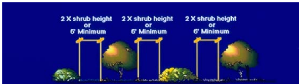
Figure C-16. Create horizontal spacing between trees and shrubs by removing shrubs from around trees within a radius that extends 3 feet from the tree's drip line. For trees taller than 6 feet, remove shrubs within a distance of 6 feet from the tree's drip line.
