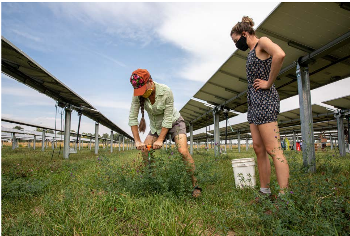
Figure 6. Soil sampling to understand soil characteristics of an InSPIRE agrivoltaic site.
