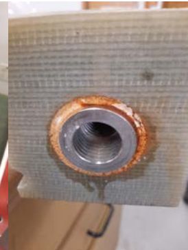
Double-Ended-Insert – metal/composite interconnect
