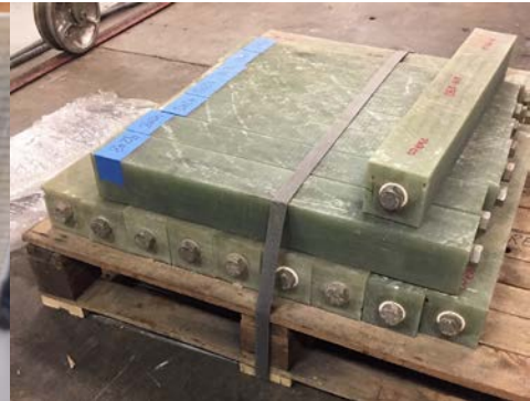
Double-Ended-Insert – metal/composite interconnect
