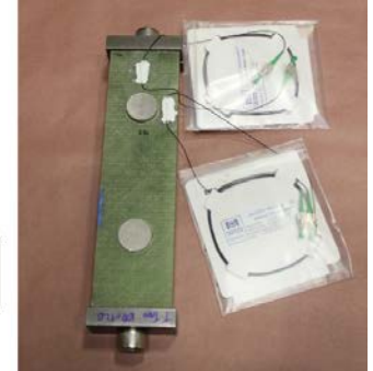
T-Bolt – metal/composite interconnect
