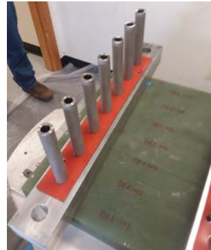
Double-Ended-Insert – metal/composite interconnect
