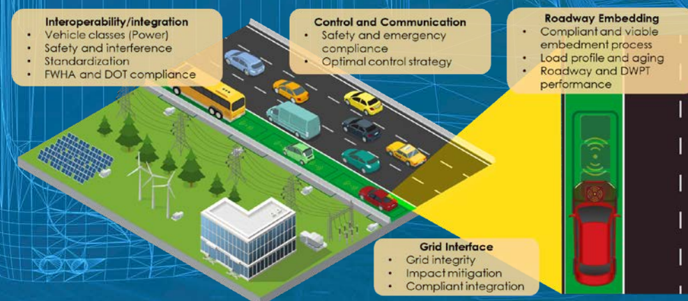
Considerations for at-scale deployment of high-power DWPT system
