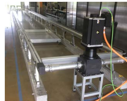
Laboratory validation of 200 kW DWPT Planned 200 kW 55 mph DWPT validation using dynamic inductive charging emulator at ACM
