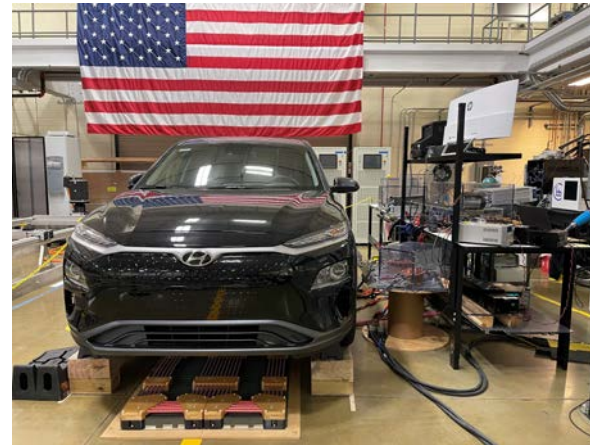
200 kW DWPT system with the receiver coil mounted on Hyundai Kona
