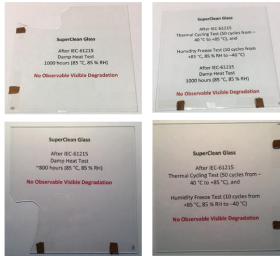
Figure 7. Images of samples after different durability tests.
