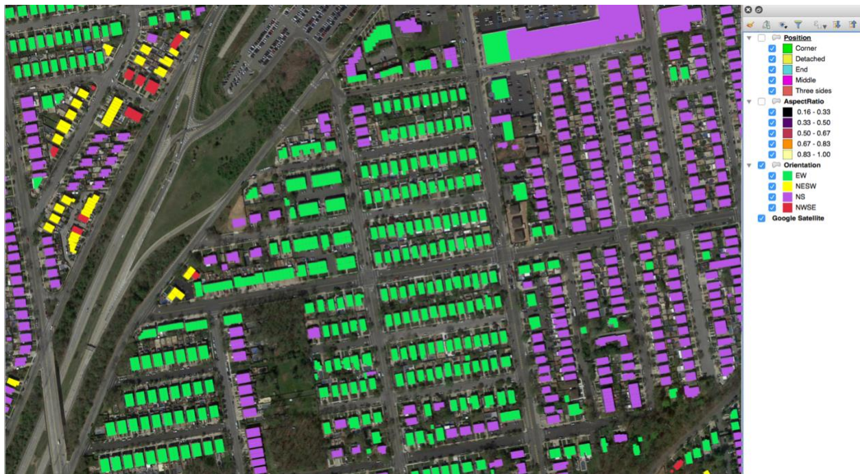
Figure 4. Building geometry input probability distributions were derived from OpenStreetMap data. This example shows building footprints being categorized by orientation of the footprint's long axis.
