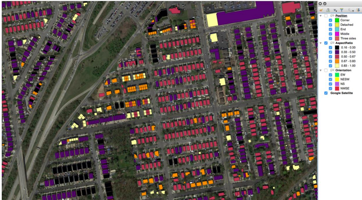
Figure 3. Building geometry input probability distributions were derived from OpenStreetMap data. This example shows building footprints being categorized by footprint aspect ratio.
