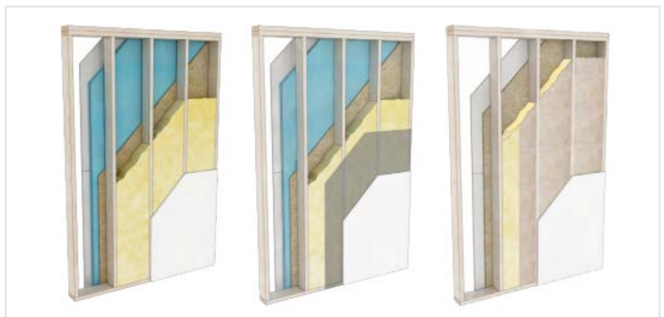
Wall configurations studied include continuous insulation and cavity insulation (no dedicated interior vapor retarder; temperature-controlled cavity) (left); continuous insulation, cavity insulation, and an interior vapor retarder (hybrid wall) (center); and cavity-only insulation (vapor-open walls or walls with an interior vapor retarder) (right).
