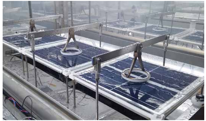
Combined accelerated stress testing (C-AST) chambers can subject PV modules to heat, cold, moisture, UV, current bias, and mechanical stress, often simultaneously. Photo by Peter Hacke
