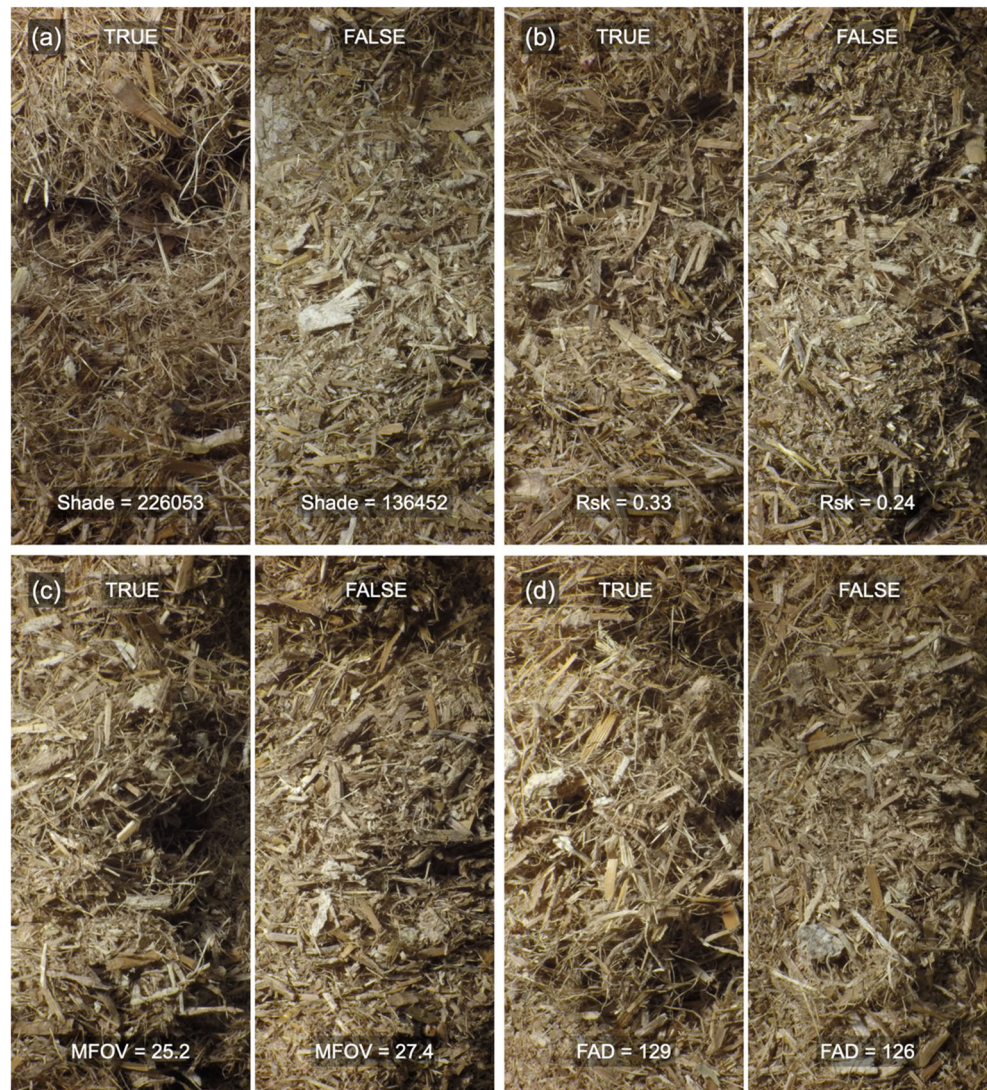
Fig. 8 Examples of feedstock images from the central one-third of the field of view. These images show the morphology of the biomass pile in the conveyor belt when it classified as TRUE or FALSE. Images with median values for the textural parameters shade (a), Rsk (b), MFOV (c), and FAD (d) are shown, all of which had a positive correlation with increased likelihood of a strain on the cross-feeder
