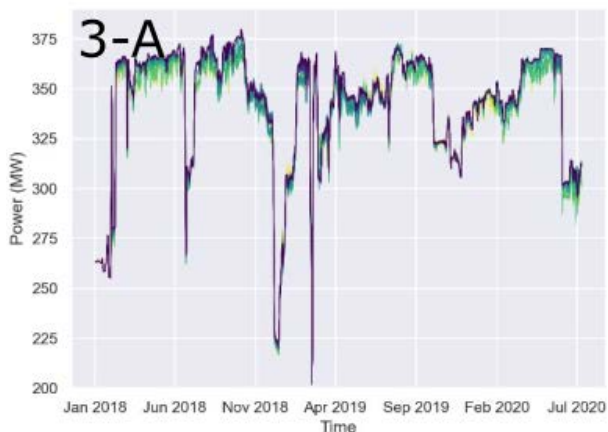
Figure 9: Results of Reinforcement Learning Experiments. Experiment 1 was not successful and was unable to achieve a greater overall output as the reward was set too low. Experiments 2 and 3 improved system output through a reward that was centered at 100% of the total baseline output. By aiming to achieve a higher than baseline, the agent was able to successfully achieve an overall higher production from the system.
