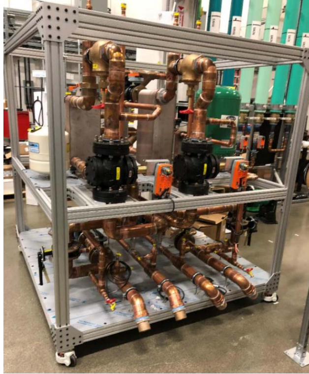
Figure 14. Pre-Fabricated Fluid Conditioning Module (FCM)
