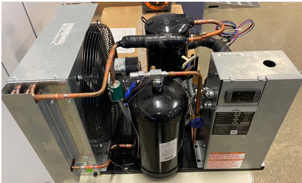
Figure 3. Baseline Condensing Unit Pre-Installed
