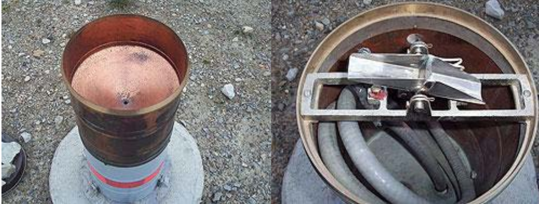
Figure 50. Tipping bucket rain gauge (left), and with the top removed to show the tipping bucket mechanism (right)
