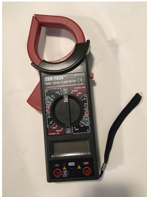
Figure 24. Example of a clamp-on CT, aka Amp Clamp
