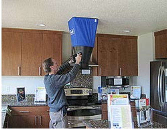
Figure 10. Passive flow hood in use at a field test site
