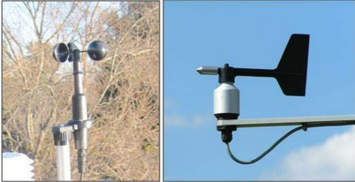
Figure 46. Three-cup anemometer at a field test site
