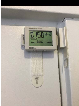
Figure 30. Example of a stand-alone door open/closed sensor/logger
