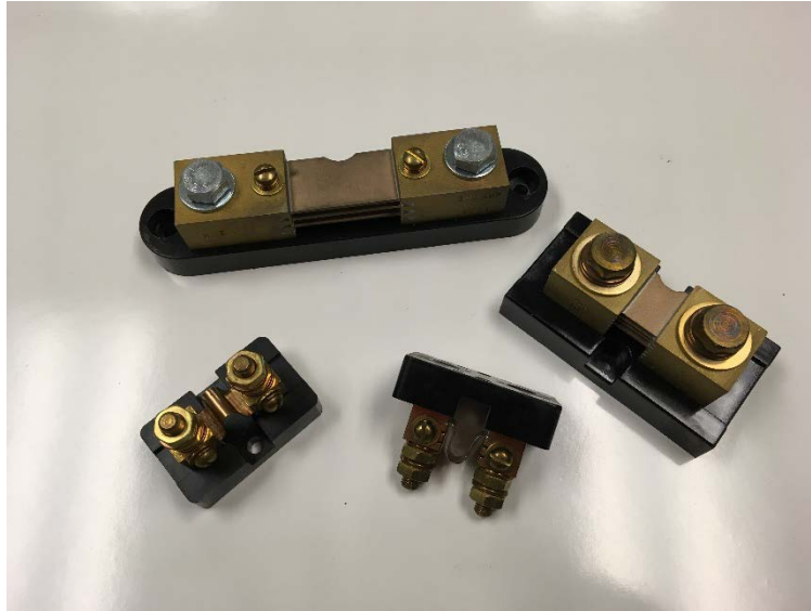
Figure 26. Shunts used for measuring DC current
