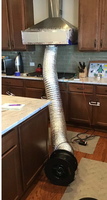
Figure 8. A kitchen exhaust fan test setup using a custom air capture box and a powered ducted fan
