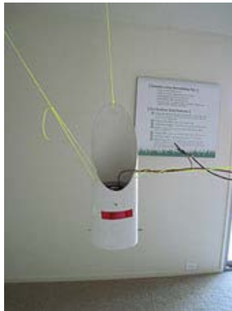
Figure 42. A custom fabricated aspirated shield in use
