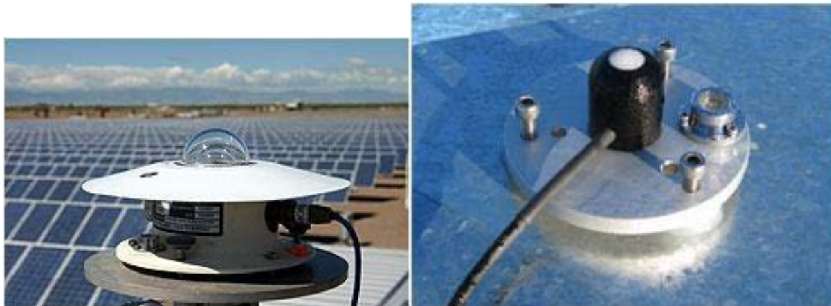
Figure 32. Thermopile-type pyranometer (left), and PV detector-type pyranometer (right)
