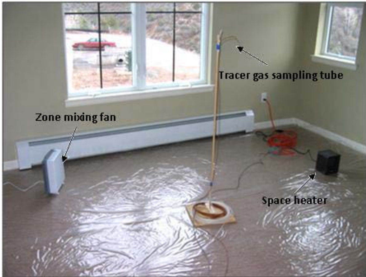
Figure 9. Tracer gas testing setup, including a space heater, a small fan, and a sampling tube
