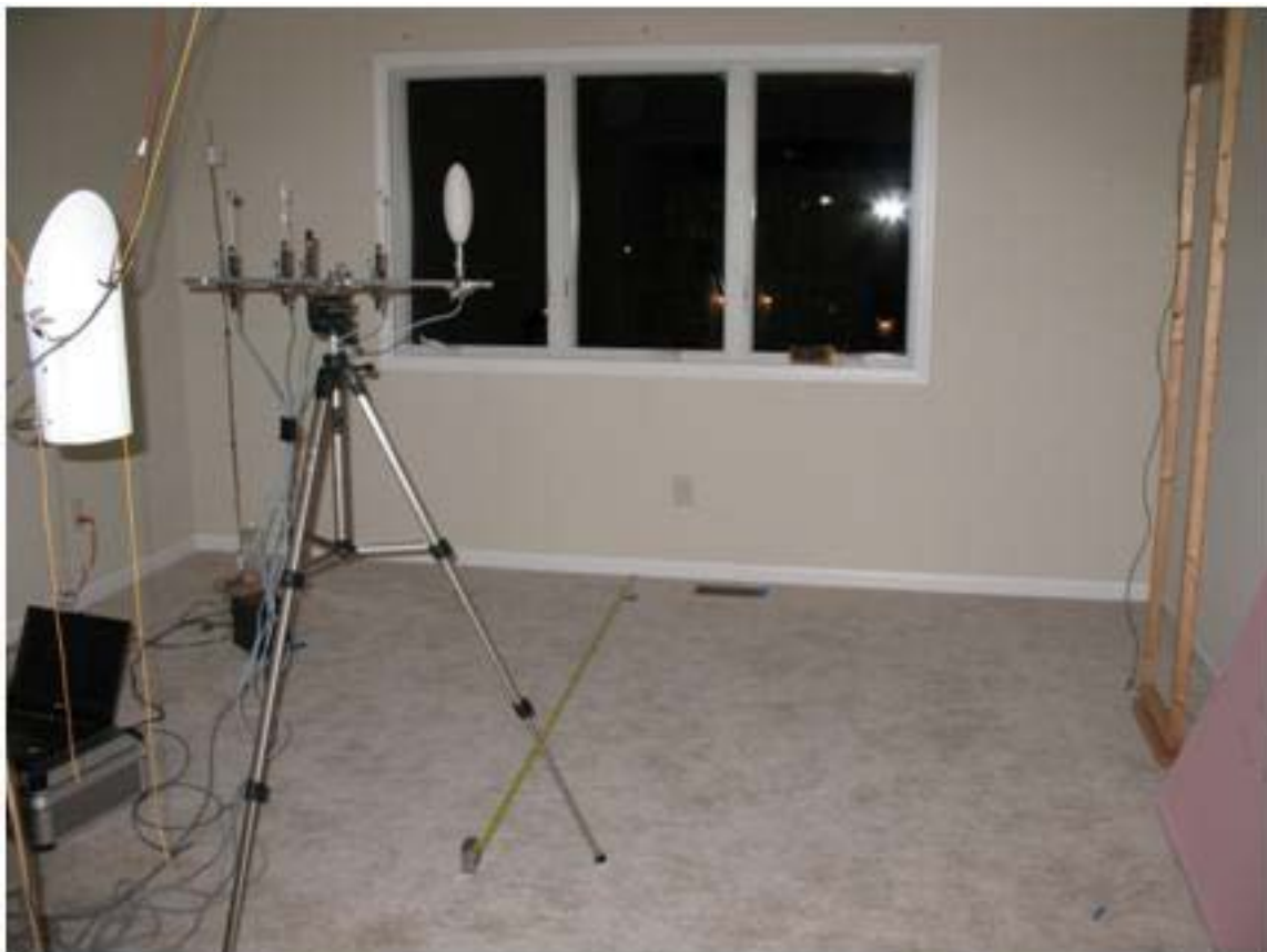
Figure 45. Thermal comfort instrument set during a field test
