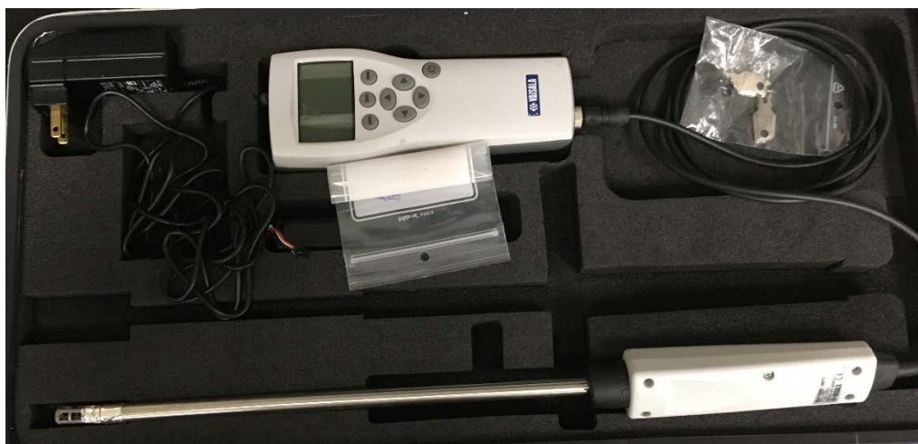
Figure 17. Additional example of a temperature and relative humidity sensor
