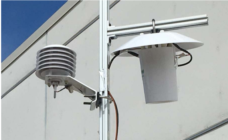
Figure 41. A commercially available passive shield on the left and a commercially available aspirated shield on the right
