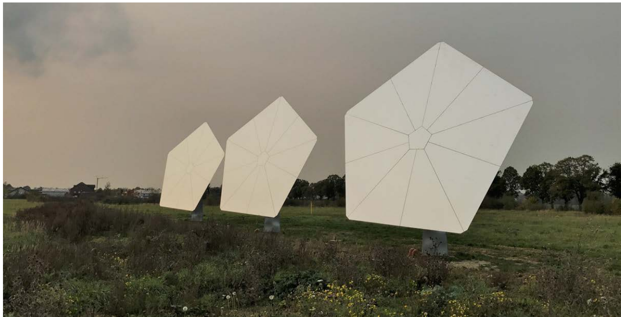
Figure 7. Installed Stellio heliostats with flat glass panels.
