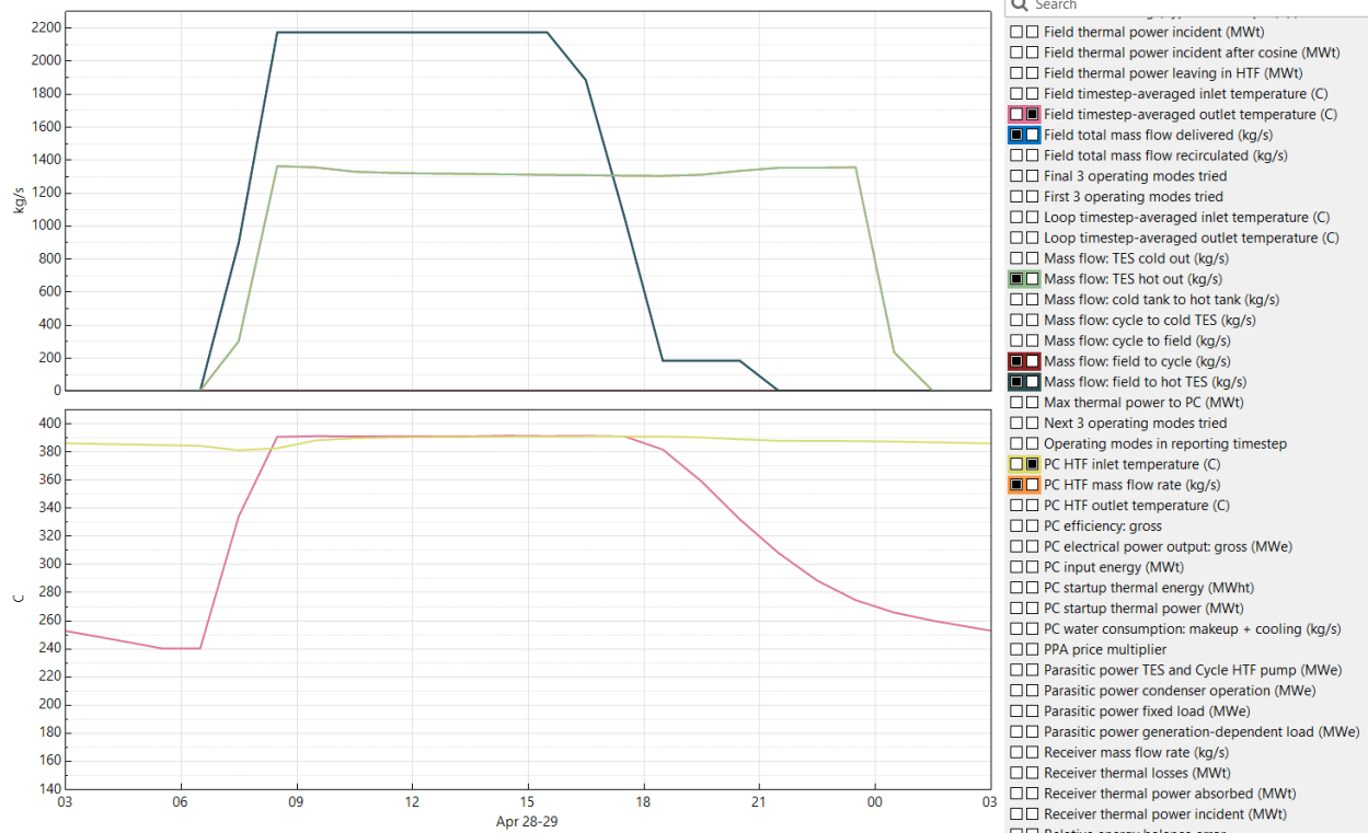
Figure 35. Temperature and flow rate of streams between field, TES, and power cycle for serial operation of the Parabolic Trough – Physical model using the decoupled configuration code.
