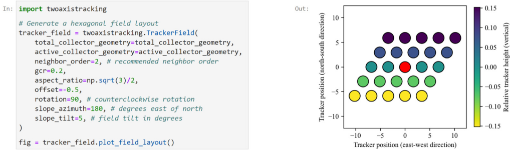
Fig. 6. Demonstration of how to use the TwoAxisTrackerField class to generate a field layout. The figure on the right shows the reference collector in red, and the neighboring collectors are colored according to the relative tracker height ( z ).
