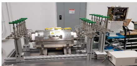
Figure 1: Multi-bed catalytic micro reactor with no heat tape or insulation
