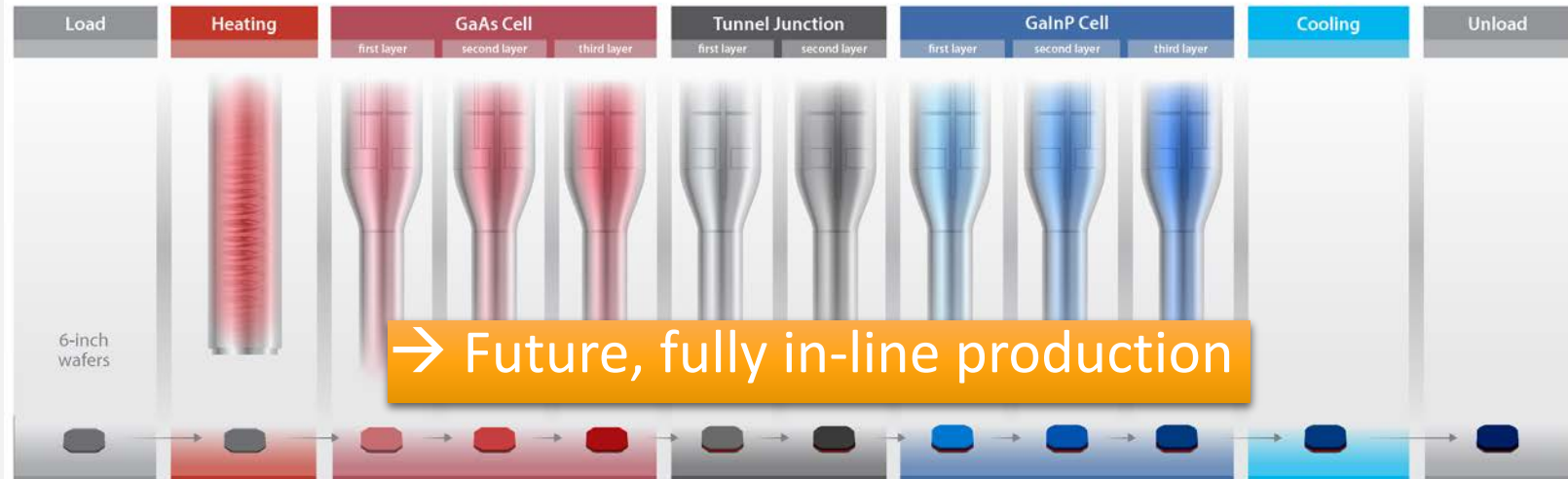
Stage 2: Throughput per tool: 75 wafers/h Production capacity: 2 MW/year
