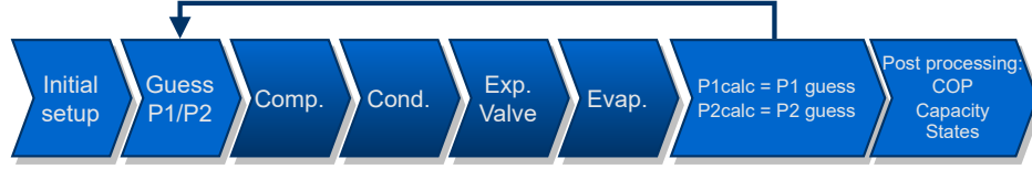
Figure 3: Vapor compression solution scheme.
